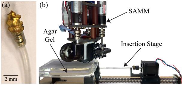
**Fig. 2** (a) Image of the tip of the needle prototype. (b) Experimental setup with the SAMM positioned above the tip of the needle in the agar gel. The needle is inserted via a robotic insertion stage.
