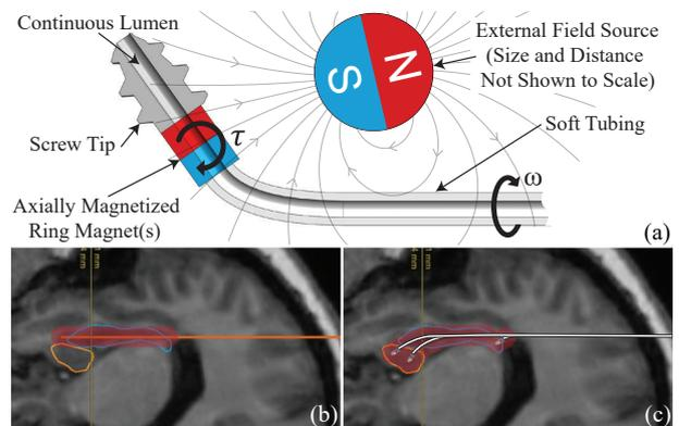
**Fig. 1** (a) Cross-section schematic of the needle concept and depiction of the field of an external permanent magnet being used to steer the needle. Our two control variables are  $\omega$  and  $\tau$ . (b) Straight needle insertion and region of ablation with sub-optimal coverage of the hippocampus (blue) and amygdala (orange). (c) Steerable needle insertion and possible region of ablation with three branching paths that more closely follow the shape of the hippocampus and amygdala.
